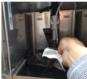
Clean the top piston with a wet cloth
