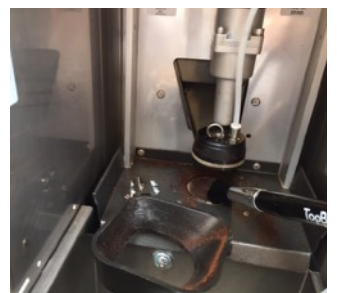
Remove dry coffee with a soft brush.
