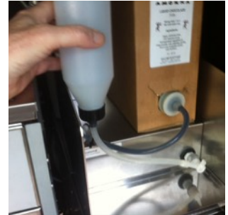
Connect the rinse bottle and open the tap.
