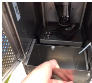
Lift out the dreg bin and empty.
